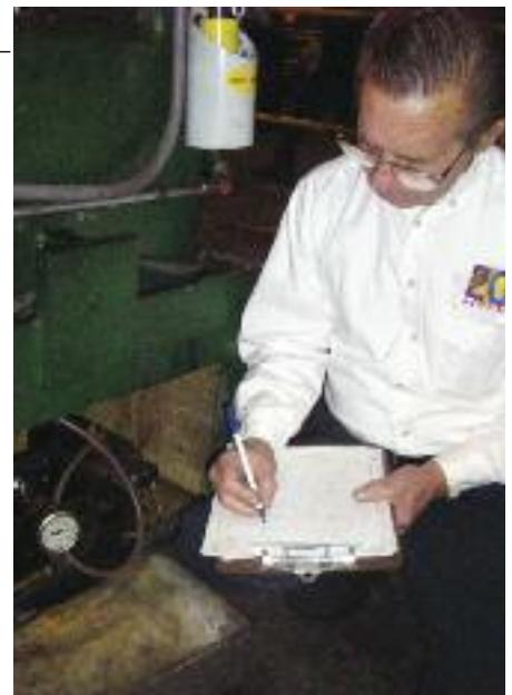
Talan's Gene Sawyer takes an hourly reading from a press's oil-pressure gauge. As part of the firm's directive to implement a "visual factory," it replaced its previous gauges with larger gauges, and repositioned them to allow easier and more accurate readings.
