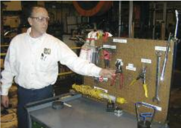
Talan Products' supervisor Frank Lowe grabs a tool off one of the firm's die carts designed as part of the firm's recent 5S and quick-die-change initiatives.
